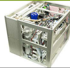
Water Recovery System
